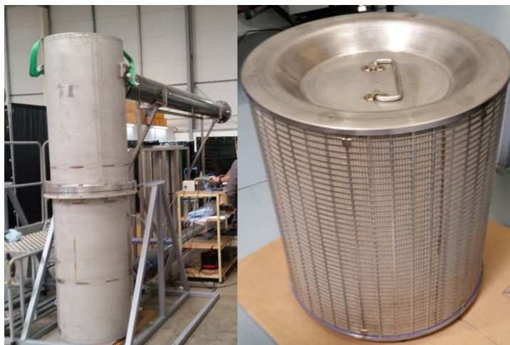
Fig. 2. Full-Scale 3400\text{ m}^3/\text{hr} (2000 cfm) Air Flow Rig, Porvair UK (left) and Porvair Radial Flow HEPA (right).
